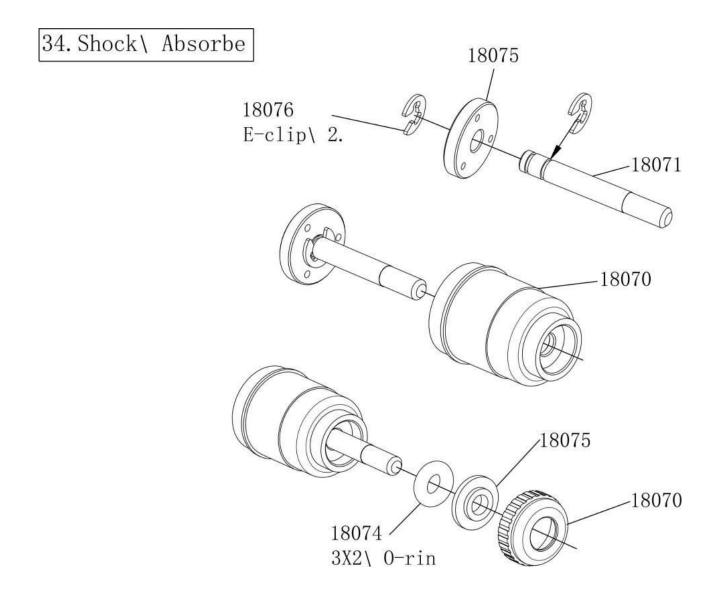
To make shock absorbers work best, it is recommended that to use 3.2x5x0.2mm shims between the O-Ring (CSO-18074) and the stem plastic washer (CSO-18075).
