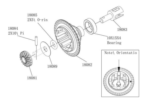
In order to have a smoother and sliding differential is suggested to replace washers in the differential coded by CSO-18089 5x15 0.4mm thickness, with 5x15 washers 0.2 thickness or less.
