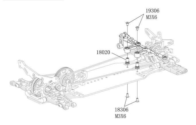
To eliminate vertical play on the postponement of the steering insert a 5x7x0.2mm shim, not included in the kit, between the studs (part number 18020-CSO) and the reference steering (CSO code-18019).
